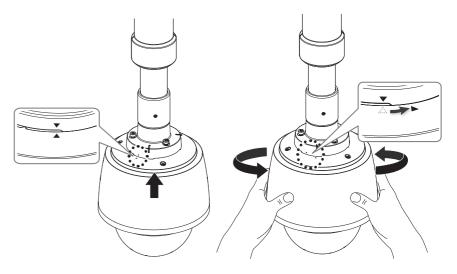
6. Tightly fasten the 3 mounting screws on the top side of the mount.
