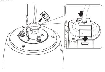
After aligning the installation direction guides of the camera and wall & pole mount, push the main cover upward and turn it counterclockwise until it is secured.
