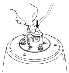
The length and width of the cable bushing are different. Check the shape and plug it in the right direction.
