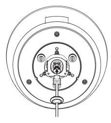
3. Plug the cable bushing of the network cable in the hole.
