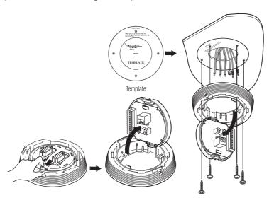
In the case of installing the camera at highly humid place, install it on the ceiling after attaching the enclosed insulation sheet on the back of install base.
