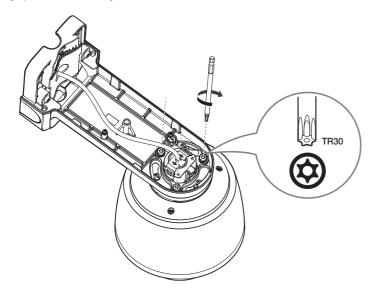
7. Join the top cover of the wall & pole mount.
