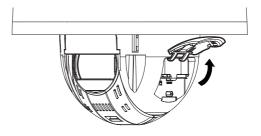
3. Insert Micro SD cards in the direction of the arrows as shown in the figure.
