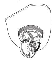
Do not connect the camera to a power outlet until the installation is complete. Supplying power while the installation is in progress may cause fire or damage the product.
