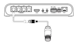
Turn off the camera power when connect or remove lens module.
