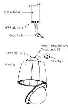
4. Install on the pipe by turning the housing in a clockwise direction, referring to the figure below.
