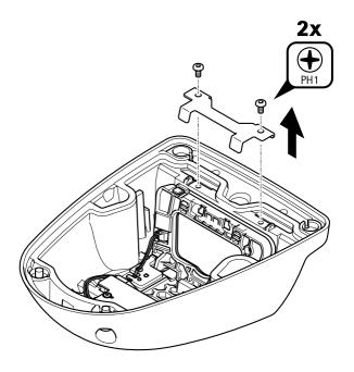
2. Remove the two screws and the bracket.
