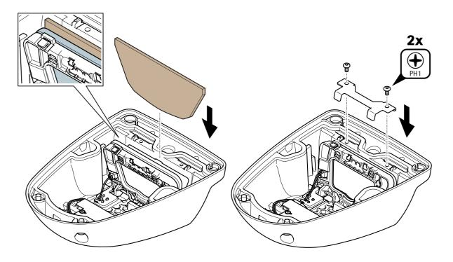
1. Mask the front window with the included cardboard. Make sure the cardboard is properly positioned. Reassemble the bracket and fasten the two screws.
