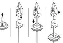
4. Insert the cable bushing into the groove of the housing installation unit.
