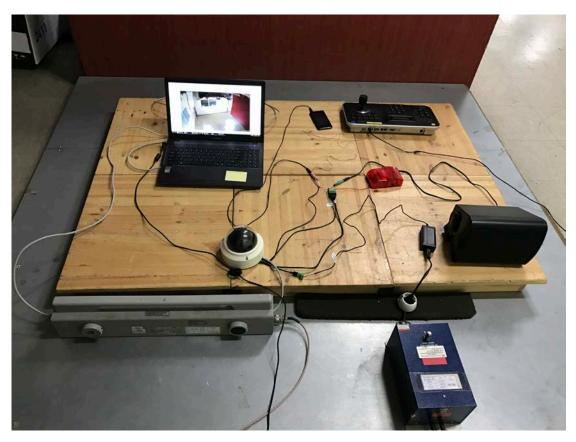
Conducted Disturbances, Induced by Radio-Frequency Fields / Capture mode (PoE)
