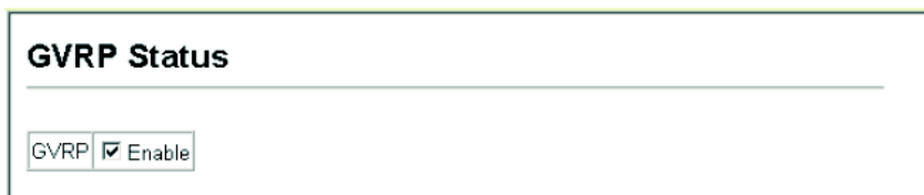
Figure 3-106 Globally Enabling GVRP
