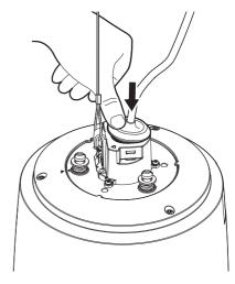
■ The length and width of the cable bushing are different. Check the shape and plug it in the right direction.
