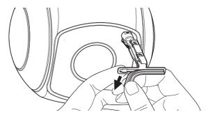
4. Insert the rubber replacement in the joint groove by sliding it in the direction of the arrow.
