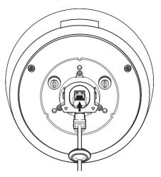
4. Plug the cable bushing of the network cable in the hole. When plugging it in, press the whole bushing area evenly so that it is properly plugged in.
