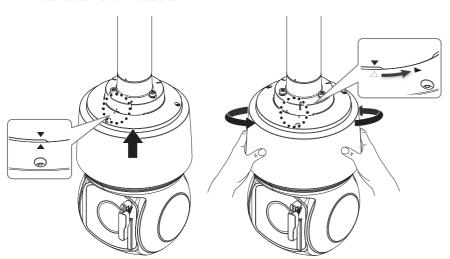
7. Tightly fasten the 3 mounting screws on the top side of the Hanging Mount.
