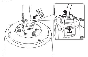
5. After aligning the installation direction guides of the camera and wall & pole mount, push the main cover upward and turn it counterclockwise until it is secured.
