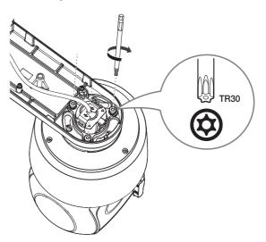
7. Join the top cover of the wall & pole mount.
