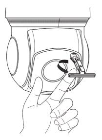
3. Remove the rubber part by pulling it back.
