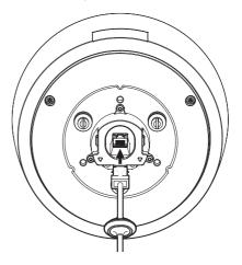
Plug the cable bushing of the network cable in the hole.When plugging it in, press the whole bushing area evenly so that it is properly plugged in.
